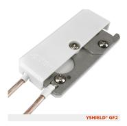
Medium-sized surface/flush mounting housing 40x80 mm, for the installation directly on shielding products or for clamping the grounding straps. With a clamping point for grounding straps preferably for small surfaces with shielding paint, shielding mesh, shielding plaster, reinforcement fabric. Usage on the interior as well as the exterior (additional seal necessary). One piece is needed per surface. Flush mounted with a height of 11 mm is thinner than a drywall construction board.
